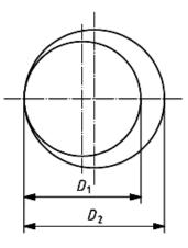
a) Radial clearance,  $C_R = R_2 - R_1$
